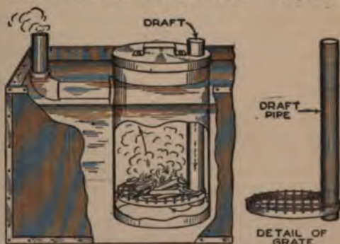
Water-Trough Heater: This Simple Device will Prevent the Water from Freezing in Cold Weather. Wood or Coal may be Used as Fuel
